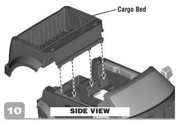
• Fit the cargo bed onto the back of the vehicle as shown. The four tabs on the cargo bed should fit into slots in the vehicle.
